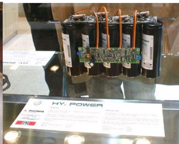
Double Layer Capacitors (Adsorbed layers of ions and solvated ions)
