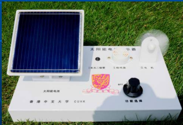
Champion solar mini-module: 10\text{cm} \times 10\text{cm} (non-gridded)
